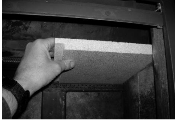
Figure 16 (cont.) - Removing/Replacing the Baffle for Inspection
