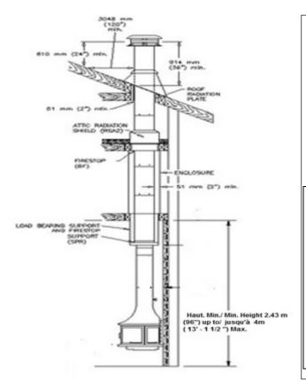
TYPICAL CONNECTION OF A BORDELET WALL-MOUNT FIREPLACE TO A PREFABRICATED 203mm (8") INTERNAL DIAM. CHIMNEY CONFORMING TO THE FOLLOWING STANDARDS: IN CANADA: ULC S-629 IN THE U.S.A.: UL 103HT
