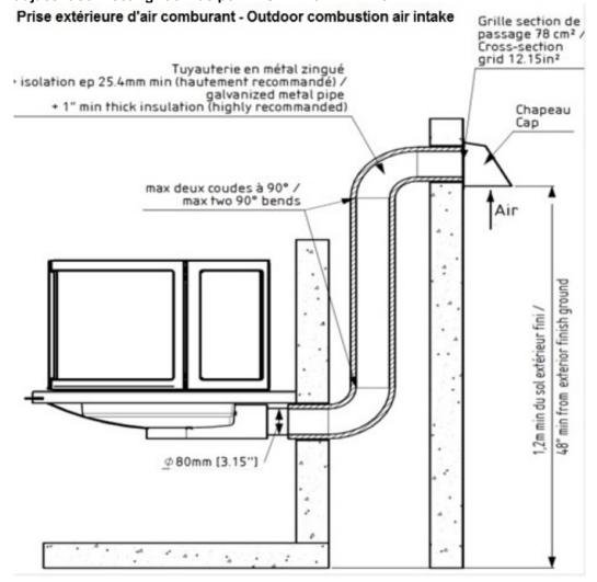
Caution: the Outside Combustion Air intake must not come from an attic, garage, carport, basement, the chimney's enclosure or be less than 3m (10') from a gas meter, a fuel/propane tank or any other device that may emit fumes or gases, such as the exhaust of a motor vehicle.
