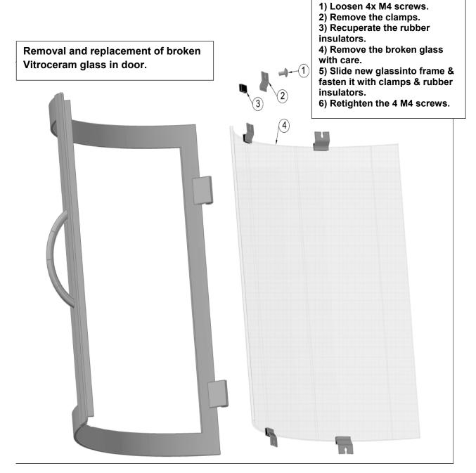
Follow these steps to install or replace the glass in Vitroceram fixed panels of a Lea 998 fireplace: (N.B. --For a new installation, start at step 6 and <u>always use protective gloves to handle glass.)</u>
