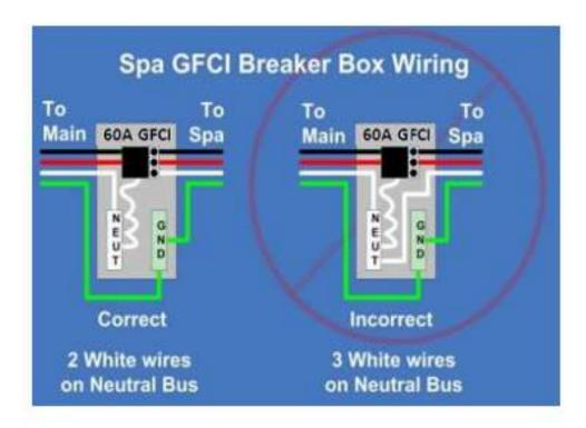
IMPORTANT: Use only a GFCI Circuit Breaker (Siemens or similar). Installation, including selection of conductor size and type, must be performed by a qualified electrician in accordance with the National Electrical Code or the Canadian Electrical Code, and all federal, state and local codes and regulations in effect at the time of installation.
