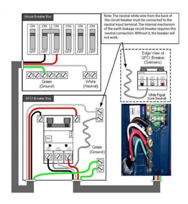
Figure 3 – Cable schematics
