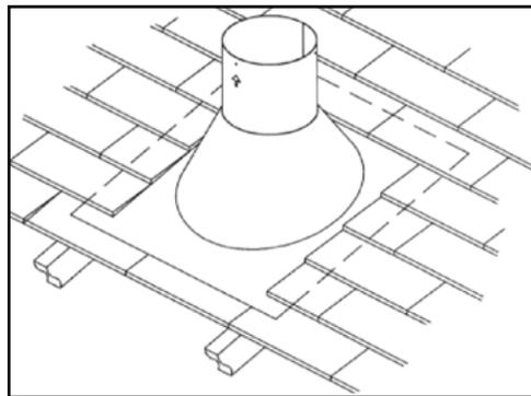
Figure 10.0.04: Flashing Installation
