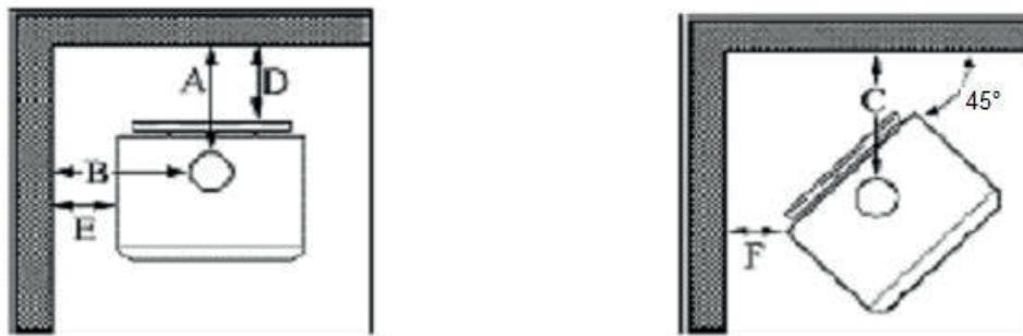
Figure 4. a) Parallel installation, b) Corner installation
