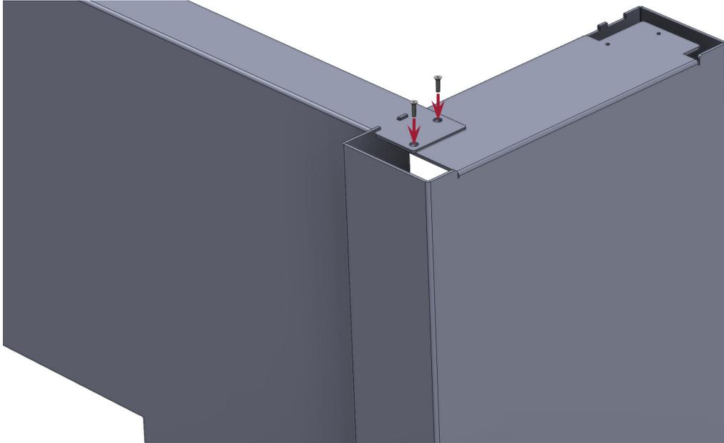
Attach the rear mounting bracket (e) to the top of the vertical supports. Insert the cleats through the corresponding slots, and secure in place with the provided self-tapping screws.
