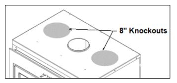
Figure 3-18: 8 Inch Knockouts for Gravity Kit
