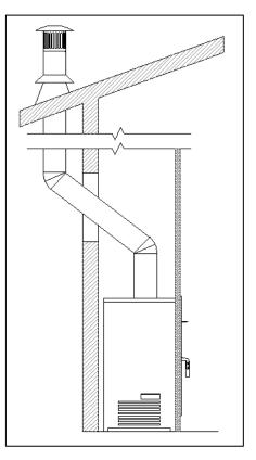
Figure 3-6: Exterior Installation
