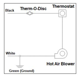
Figure 4-4: Electrical Diagram for Hot Air Kit
