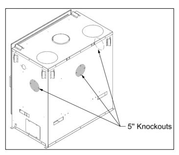
Figure 4-2: Hot Air Kit Knockouts
