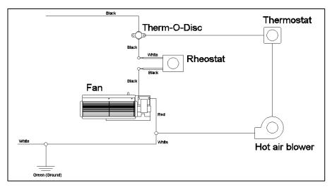
Figure 4-3: Electrical Diagram for Parallel Connection of Hot Air Kit and Blower Kit
