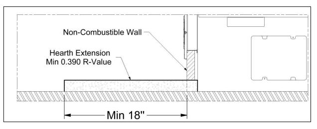
Figure 3-25: Hearth Extension Extended to Unit
