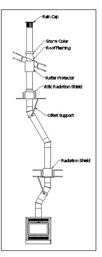
Figure 3-7: Offset Installation
