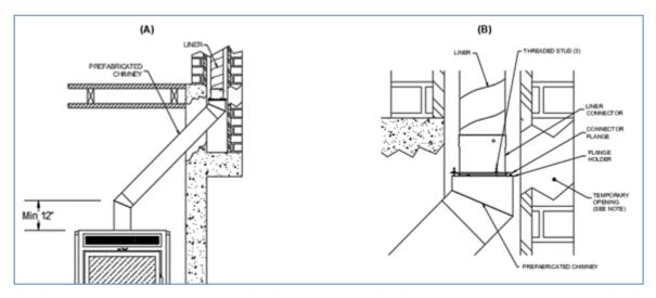
Figure 3-9: (A) Connection into a masonry chimney through an elbow/liner; (B) detailed drawing of masonry chimney connection.
