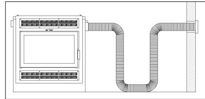
Figure 4-5: Installation of Fresh Air Kit
