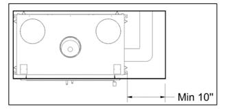
Figure 3-4: Space Required for Fresh Air Kit Installations
