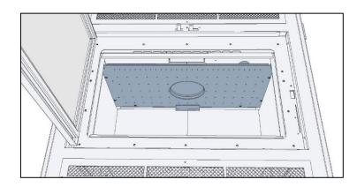
Figure 2-10: Baffle Secondary Burn Technology
