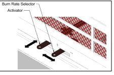
Figure 2-5: Combustion Air Control's Activator and Burn Rate Selector
