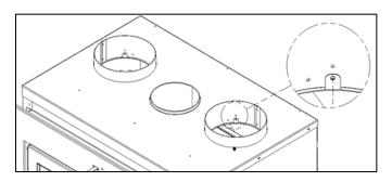
Figure 3-20: Tabs Inside the 8 Inch Knockouts
