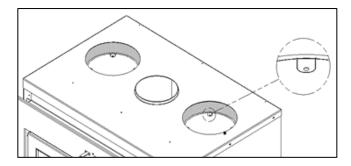
Figure 3-19: Tabs Inside the 8 Inch Knockouts
