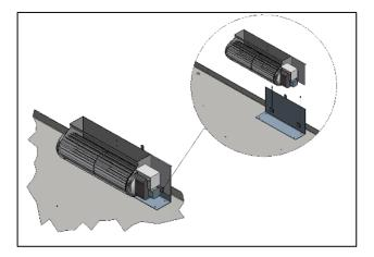
Figure 3-32: Blower and its Fixture
