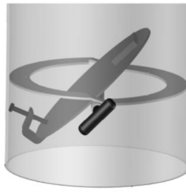
Fig. 1: Proper installation of damper stop.
