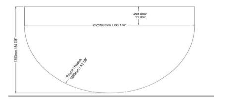
2.2.3 Installing the extension pipe(s), the ceiling cover plate and the Fireplace on the
