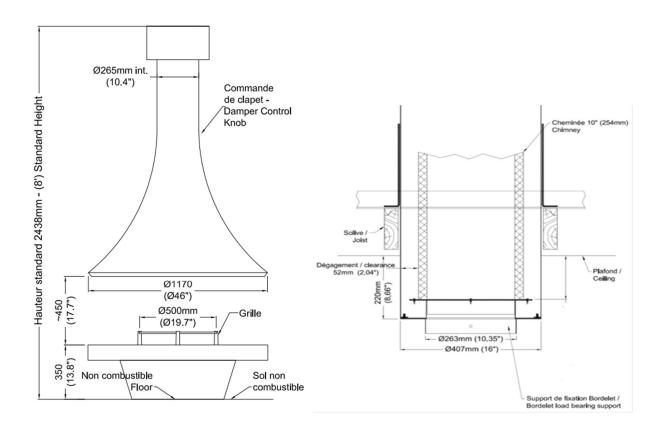
Warning: For centrally-located fireplaces, a minimum clearance to combustibles of 1.2m (48") must be maintained 360 ° around the fireplace. For single wall smoke pipe, a minimum 45cm (18") clearance to combustibles must be maintained and, when connected to the Bordelet Load Bearing Support, a minimum 220mm (8- 11/16") clearance from the top of smoke pipe mounting flange to the ceiling must be maintained, especially with slanted ceilings. Adjust the height of the Load Bearing Support accordingly.
