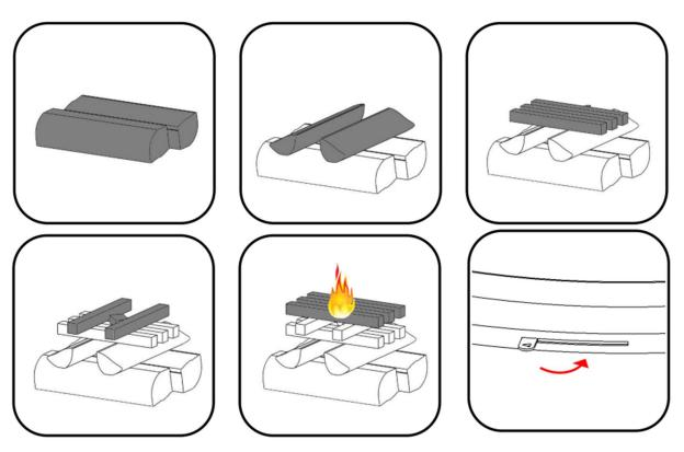
REMINDER: The ignition of the appliance must be carried out using this ignition method (reverse ignition).
