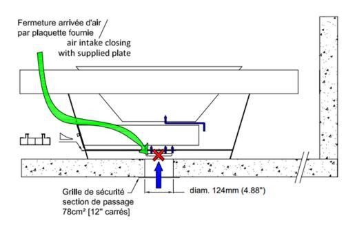
Caution: the Outdoor Combustion Air intake must not come from an attic, garage, carport, basement, the chimney's enclosure or be less than 3m (10') from a gas meter, a fuel/propane tank or any other device that may emit fumes or gases, such as the exhaust of a motor vehicle.
