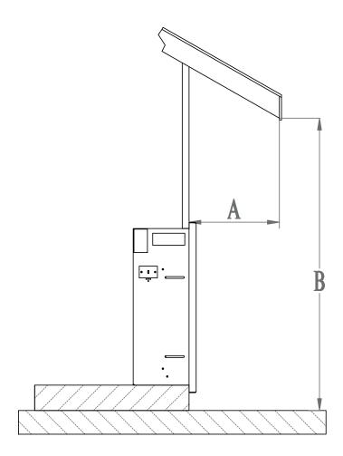
The overhang (A) must extend at least 1/2 the roof-line height. Height is measured from the base of the fireplace.
