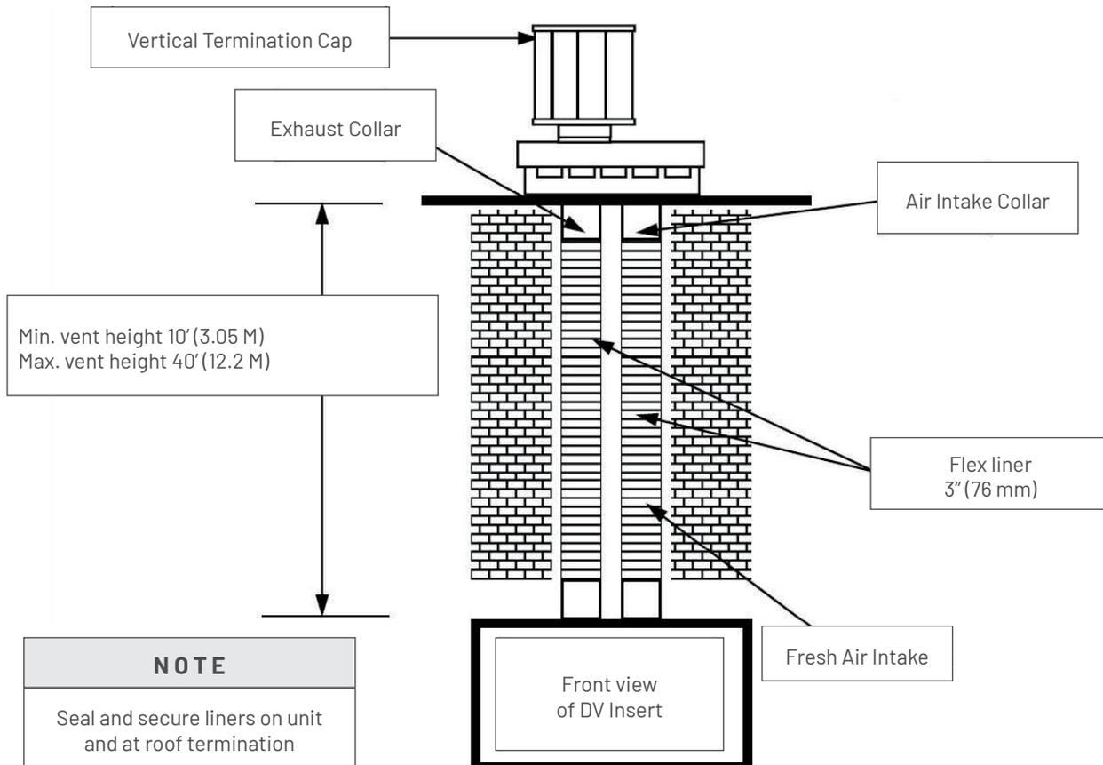
The minimum flue (chimney) size required to run the two 3" (76 mm) is 4" x 7" (100 mm x 178 mm).
