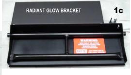
STEP 1: Figure 1a illustrates how the radiant glow bracket slides and rests on the back of the burner pan. For installation on burner pans without pilots center the bracket on the back of the burner pan as shown in figure 1b. For installation on burner pans with a pilot install the bracket on the back of the burner pan allowing 1" clearance around the pilot assembly as shown in figure 1c. The grate can then be pulled forward over the burner pan, as shown in figure 1e.
