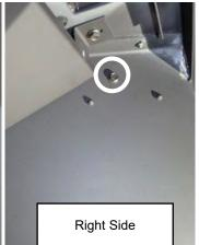
Step 2: Remove the three (3) 1/4" Tek Screws securing the masking plate at the back of the firebox.
