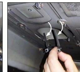
Step 2: Pull the restrictor flap from the opening.
