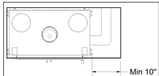
Figure 3-4: Space Required for Fresh Air Kit Installations
