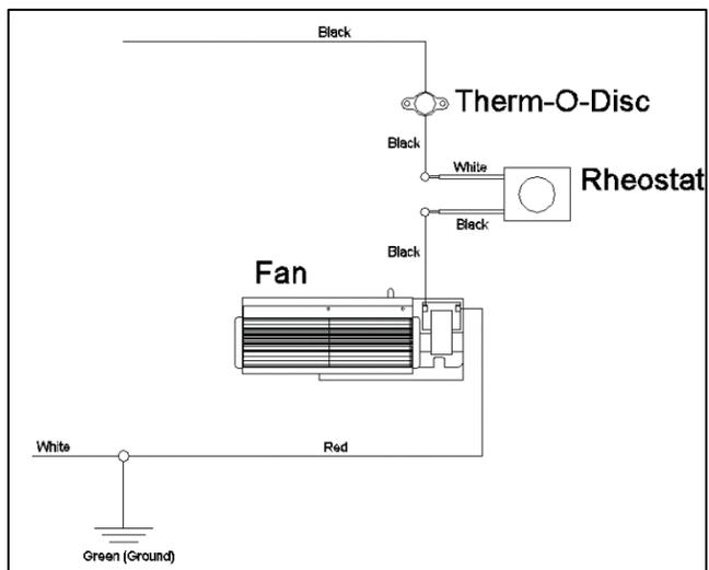
Figure 3-30: Electrical Diagram
