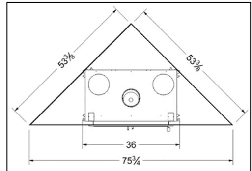
Figure 3-2: Corner Installation
