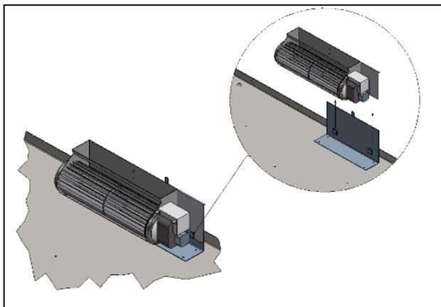
Figure 3-32: Blower and its Fixture
