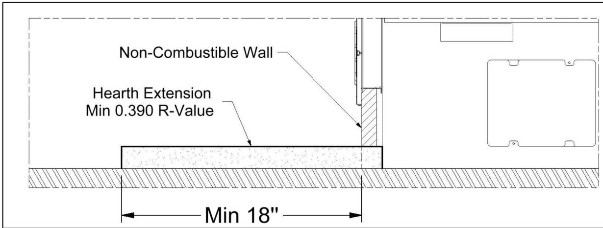
Figure 3-25: Hearth Extension Extended to Unit
