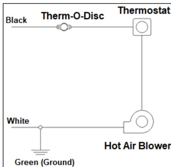
Figure 4-4: Electrical Diagram for Hot Air Kit
