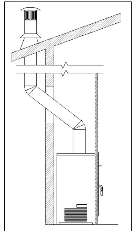
Figure 3-6: Exterior Installation
