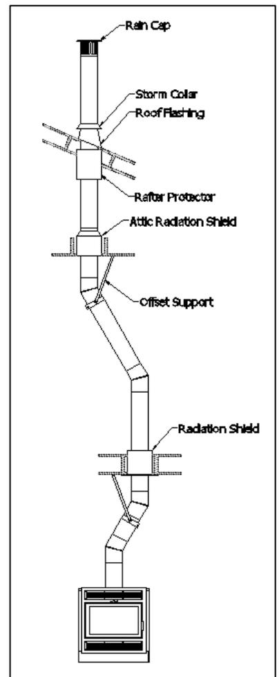
Figure 3-7: Offset Installation
